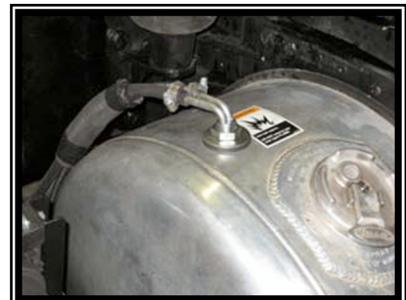
system and moving components. Fuel lines must be run along the frame side rails or under carriage.
